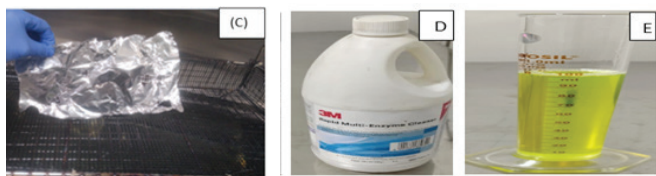
C) Foil testing after the hot water rinsing of implants. D) Cleaning Solution (3M Multi Enzymatic Cleaner). E) Cleaning Solution tube
